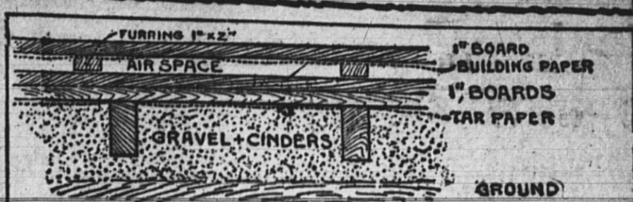
Floor and Foundation of Storage Plant.
